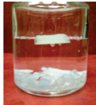
Figure 4. Hydrophobic polycyanoacrylate–silica nanocomposite aerogels float in water while unmodified silica aerogels adsorb water wet, burst into fragments and sink to the bottom of the container.
