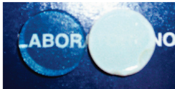
Figure 1. Photograph of uncoated aerogel (left) and of polycyanoacrylate coated aerogel (right). Monolith is homogeneously opaque. Aerogels are 0.9 cm thick and 3.5 cm in diameter.
